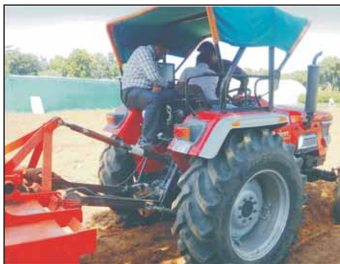
Tractor Data Acquisition for field power and energy demand mapping
