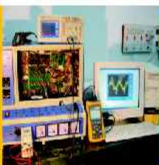
DSP Based Three Phase Matrix Converter Fed Induction Motor Drive Along With Power quality Analyzer and DSO
